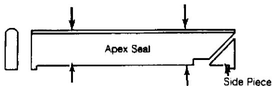
Fig. 14: Measuring Apex Seal Height Clean thoroughly before measuring.
